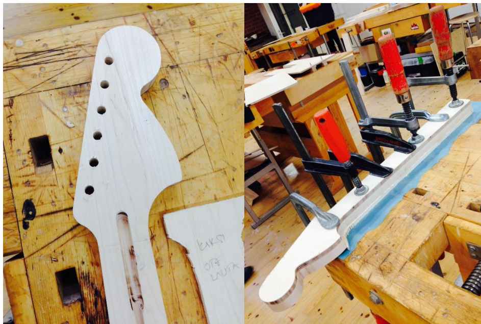
Pictures 7 and 8. Tuning machine holes and glueing the fingerboard.
