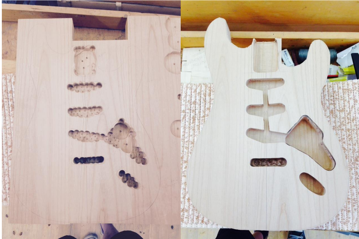
Pictures 3 and 4. Making room for the hardware and cutting the shape.
